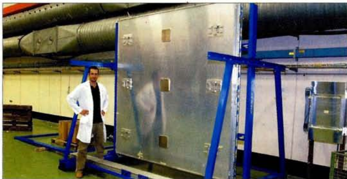
Drift-tube chambers from Spain, made for the CMS barrel muon detector, are tested and then stored at CERN.
