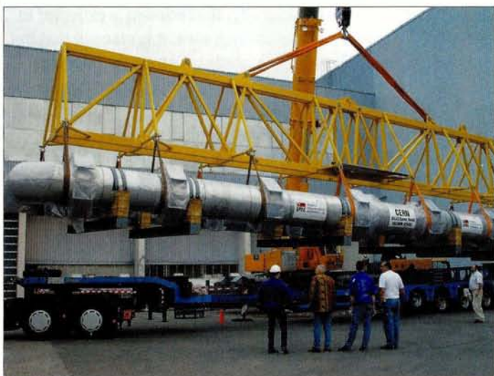
The Spanish company Felguera Construcciones Mecanicas SA has built a number of 25 m long vacuum vessels for the superconducting toroid barrel system of the ATLAS detector. Here one of the vessels arrives at CERN. (Photo: P Collins.)
