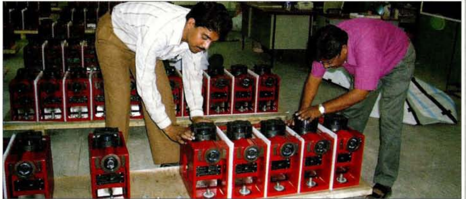
The jacks undergoing final pre-shipment inspection by engineers at CAT in India.
